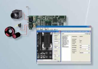
The **MultiCam driver** enables the consistent control of several Euresys frame grabbers, using an arbitrary number of cameras, from **one or several software applications**. MultiCam allows defining **channels** linking cameras to buffers in the PC memory.
